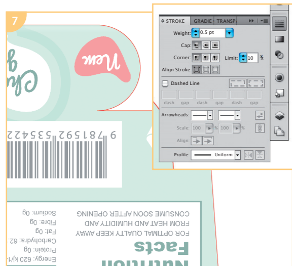
Cut lines Cut lines are indicated with solid red lines, typically .25 or .50pt.
